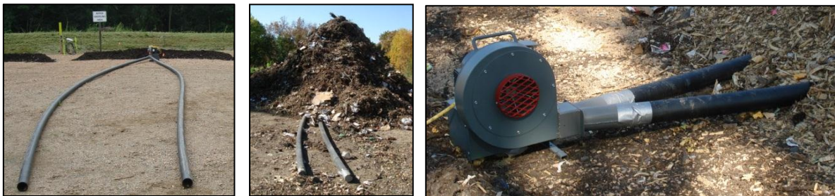
Above (left): Aeration tubes lined up on the pad. Above (middle): Aeration tubes coming out of a pile. Above (right): Blower and aeration tubes entering the pile.
