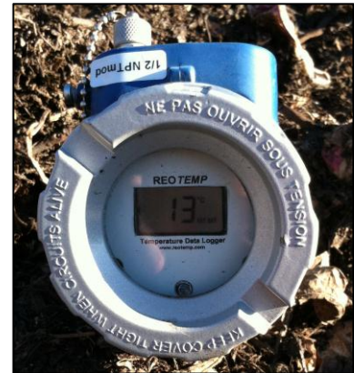
Above: Reo-Temp Compost Data Logger purchased to electronically record temperatures.
